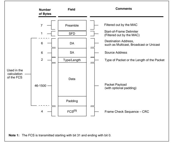
FIGURE 5-1: ETHERNET PACKET FORMAT
