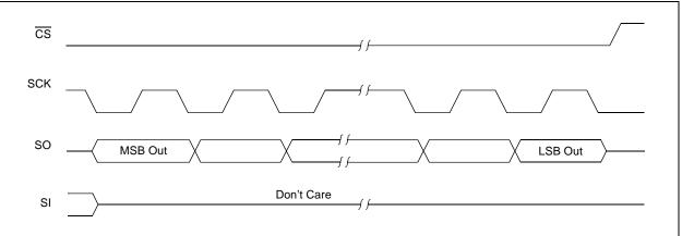
Commands and data are sent to the device via the SI pin, with data being clocked in on the rising edge of SCK. Data is driven out by the ENC28J60 on the SO line, on the falling edge of SCK. The CS pin must be held low while any operation is performed and returned high when finished.
